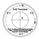
Figure 2-4 Drill Template of Junction Box
