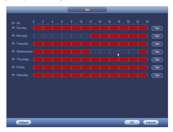
Figure 3 The period setting of alarm box
